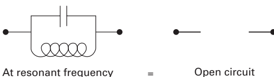
Figure 1.3. Parallel-resonant LC circuit.
