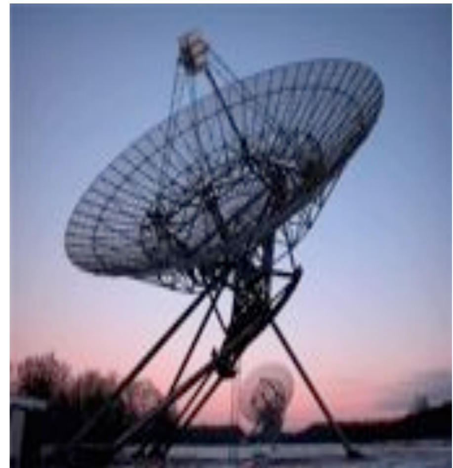
Equatorial (polar) mount
